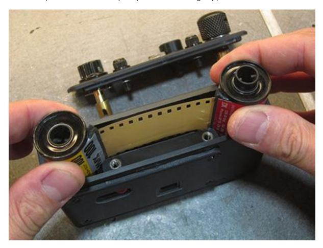
Put the clicker in place. (Ensure it is in the correct position and not stuck the cannister which can happen as cannister is made of steel).
