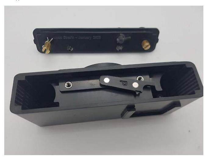
Load the film into the camera as shown (the camera lid will not fit if you try and do it the wrong way)
