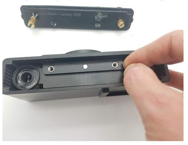
Before putting the lid on the camera ensure the dot on the 'rewind switch' is the 3 to 4 o clock position. (This puts the switch in a position to disengage the clicker for rewinding the film, if put in the wrong position it will not be possible to rewind the film in the field).
