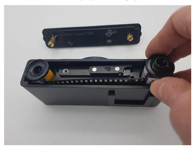
Ensure the canisters are well seated and put the clicker in place. (Ensure it is not stuck to the cannister which can happen as cannister is made of steel).
